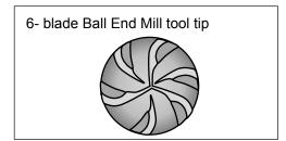
Set this function with the [Feed speed] parameter set to "Maximum number of tool edges". Set the "No. of Edges" separately for the tool tip with little edges to decelerate [Feed speed] of the tool tip. Set tool tip at [Switching angle].
