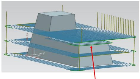
When the [Output Plane Only] function is used, the contour face cut machining path is output only for the surfaces that are recognized as planes.
