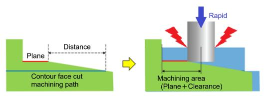
Increasing the clearance value more than necessary to increase the machining area is not recommended.
