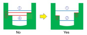
: Original contour face cut machining path
