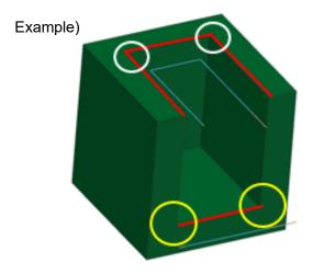
If the edges near the yellow circles are chamfered, the tool will interfere with the adjacent standing walls.
