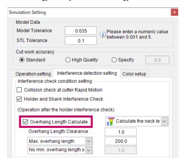
If [Overhang Length Calculate] is not selected, the values for "Overhang length (Simulation result)" and "Neck length (Simulation result)" are not included in the Excel machining information.
