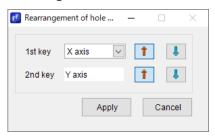
Select the axis (X or Y axis) that will be referenced by [1st key], and select the axis direction ( ascending or descending).
